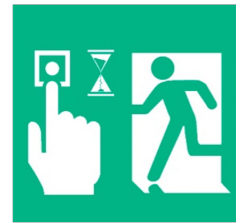
Signage for system with a time delay
